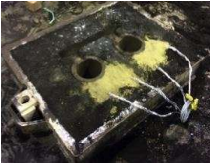
Gambar 5. Proses pengecoran 80Cr15.
